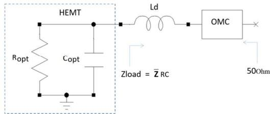
Fig.8 Equivalent RC-Circuit
