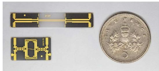
Fig.6 images of the developed quadrature couplers
