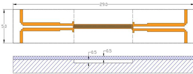
Fig.2 Design of a three-section coupler with a suspended-line central section
