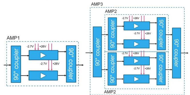
Fig. 1 Structural arrangement of pre-stage and output cascades
