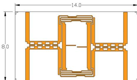
Fig.4 Topology of the new multi-cascade tandem quadrature coupler
