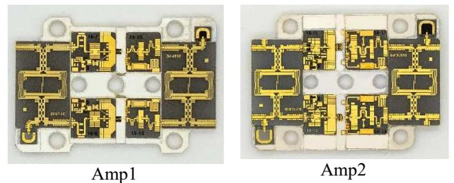
Fig.11 Images of the developed balanced amplifiers
