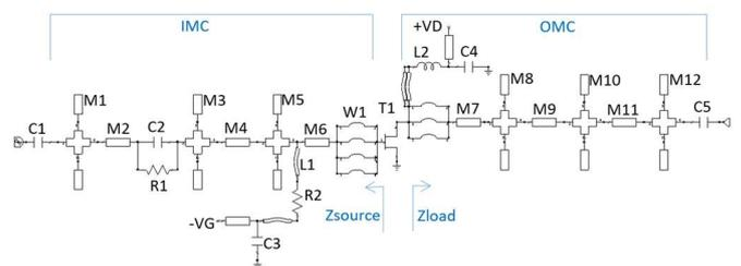
Fig.7 Structural arrangement of input and output matching circuits
