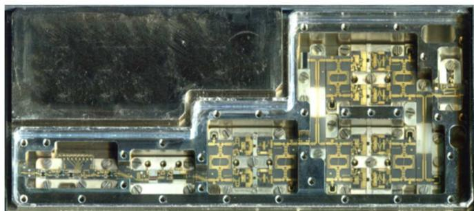
Fig.14 Layout of the amplifier
