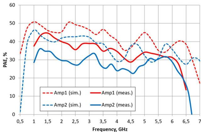
Fig.13 Simulated and measured PAE of Amp1 and Amp2
