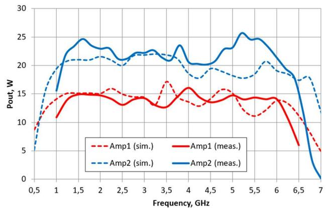
Fig.12 Simulated and measured output power of Amp1 and Amp2
