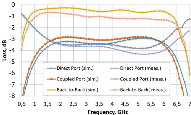
Fig.3 Simulated and measured characteristics of the 1-6 GHz three-section quadrature coupler
