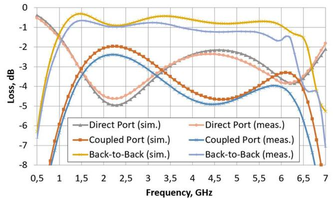
Fig.5 Simulated and measured characteristics of the new tandem coupler
