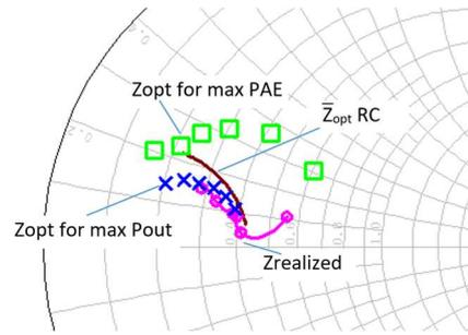
Fig.10. Realized impedance of output matching circuit Amp2
