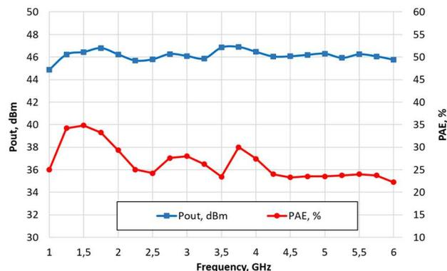
Fig.15 Measured output power and PAE at  $P_{in} = 2$  mW
