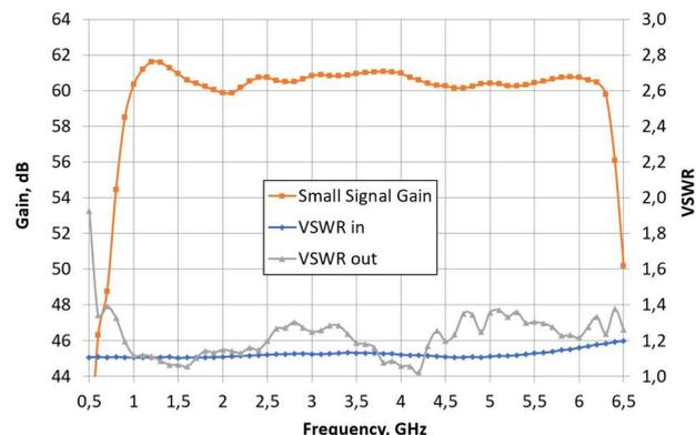
Fig.16 Measured small-signal gain and input/output VSWR
