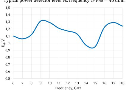
Typical power detector level vs. frequency @  $P_{out} = 40 \text{ dBm}$
