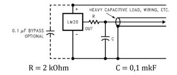
$V_{\rm O} = (-3.88 \times 10^{-6} \times T^2) + (-1.15 \times 10^{-2} \times T) + 1.8639$
